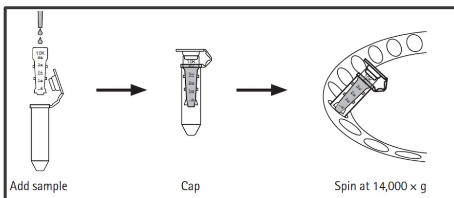
**Figure 2.** How to place the filter device into the centrifuge rotor.
