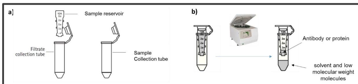
**Figure 1.** a) Protein Purify&Concentrate Kit. b) Assembly of the sample reservoir and the collecting vial.
