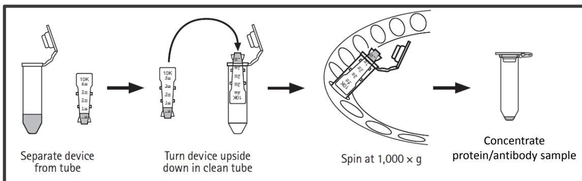
**Figure 3.** How to recover the concentrate protein/antibody sample.
