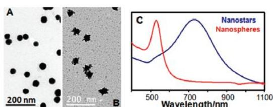
**Figure 1\_** TEM micrographs of nanospheres (A) and nanostars (B). (C) UV-vis-NIR spectra showing surface plasmon resonances of both types of nanoparticles in aqueous suspension.
