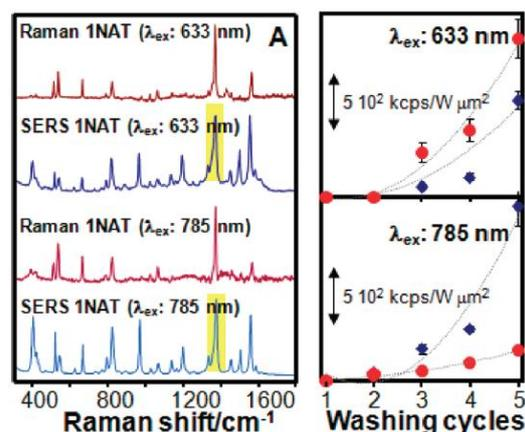
**Figure 2\_** Raman, resonance Raman, SERS, and SERRS spectra (left) and variation of the SERS/SERRS intensity as a function of the nanoparticle shape, washing cycles, and excitation laser line (right) for 1-naphthalenethiol.
